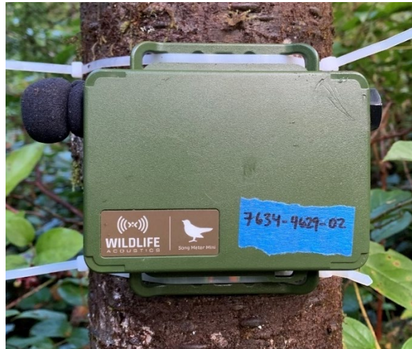
Figure 3: Song Meter Mini Autonomous Recording Unit (ARU) by Wildlife Acoustics.
