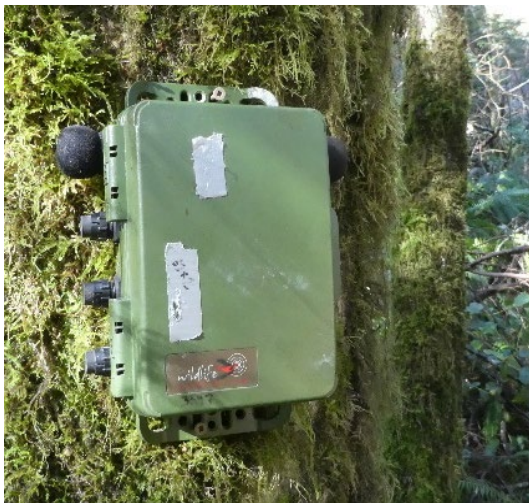
Figure 2. Song Meter SM4 Autonomous Recording Unit (ARU) by Wildlife Acoustics.
